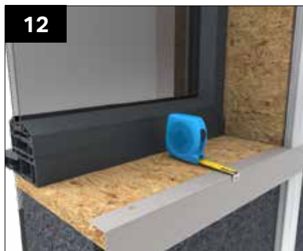
Fit windows and doors in position. The internal face of the frames (if 70mm frames are used) is to sit 70mm inboard from the external wall steel datum (or 145mm from the internal), this is the outermost steel on the top tray.
