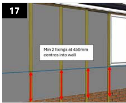
The 25*50mm treated batten running down the outer surface of the wall will be fixed to the wall at a maximum of 450mm centres using No12 screws 75mm long plugged into the wall. Now you can start to install your preferred external finish.
