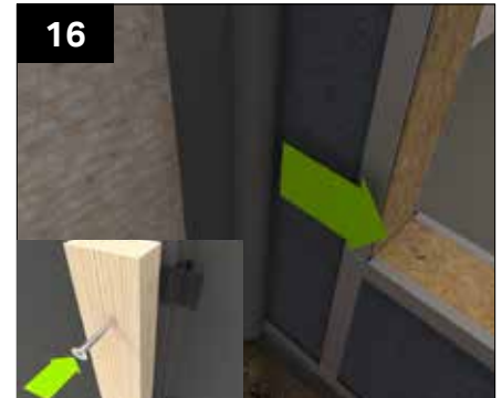
Please follow the steps within the main hup installation guide for installing the membrane and battens with the relevant roof ordered for batten positioning. Ensure the membrane overlaps onto the existing brick by min of 100mm.
