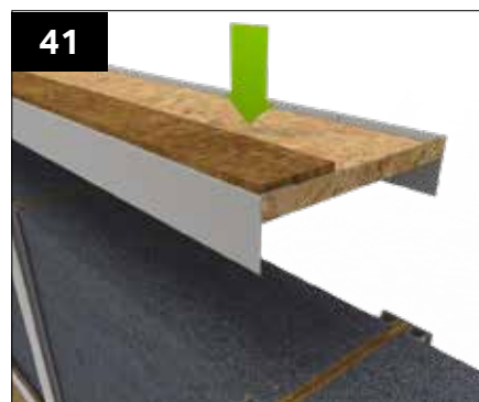
If a glass/hybrid roof has been specified top trays will be supplied. If a Flat Roof or UltraRoof has been specified, there will be no top tray. If the glass hybrid roof is specified with Cornice, the top tray will have a hardboard packer attached. This should sit towards the outside of the wall. Locate over the top of the wall panel aligning holes with clips.
