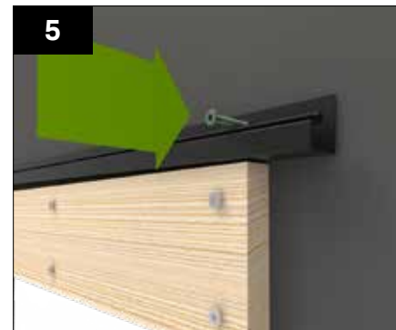
5 Fit the soaker trim to the wall at a slight angle, giving it a roughly one-degree fall. The battens should terminate above and below this trim.
