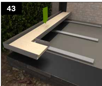
Position the base tray on top of provided steel skids. Following steps up to 12 in the general installation to position the base tray, mark this position, however do not fix down to the base at this point.
