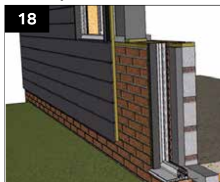
In the case where the new wall is within 1 metre of a boundary Calcium Silicate Board will be provided. This needs to be installed before battening if a cladding is being used.
